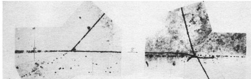
FIG. 1. A photomicrograph and schematic diagram of the production of a double hyperfragment in a 1.5-GeV/c K<sup>-</sup> meson interaction with carbon followed by capture of the  $\Xi^-$  hyperon by a nucleon and decay of the double hyperfragment into three pions.
