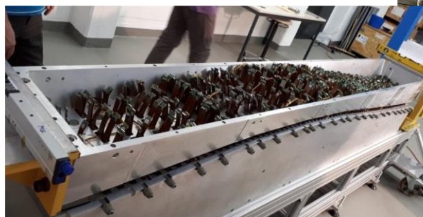
Slice of barrel calorimeter
