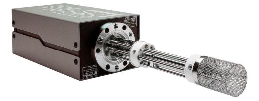
Figure 5.17: Residual Gas Analyzer RGA 200.
