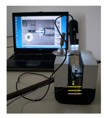
Figure 5.12: Piezo-motor performing in a magnetic field originated by a magnet with U-shape.
