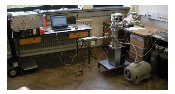
Figure 5.16: Experimental setup to measure residual gasses in high vacuum.
