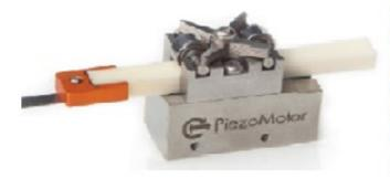
Weight: 23 g Size: 22 mm x 19.3 mm x 10.8 mm Maximum speed: 0-15 mm/s Stroke max: 80 mm Average step: 4 µm Dynamic force: 6.5 N Holding force: 7 N
