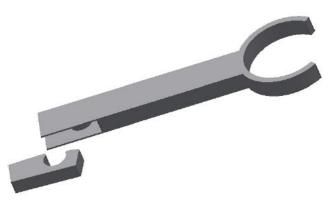
Figure 5.21: Hook designed as prolongation of the piezo-motor arm.
