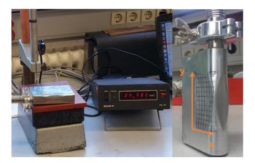
Figure 4.3: Left side: Chamber connected to the vacuum pump with the precision needle measuring its deformation. Right side: AlMg 100  $\mu$ m rounded chamber deeply deformed when pumped.
